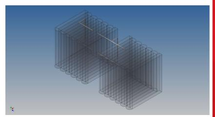
H ANCHOR MODULE Attachment can be used for standard size modules or with Macro Modules (larger size modules). This hardware system provides a strong and durable lining for longer furnace life. This attachment is quick and easy to install. The H Anchor is welded to the furnace shell and a module is slid over both sides of the anchor. Using this system, Nutec modules can only be installed in a Uni-directional pattern with batten strips.
