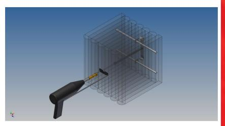
WELD-TITE MODULE Attachment is a speed weld system that requires no stud pattern or furnace layout. The advantage to this attachment system is the speed of installation. Just fire the speed weld gun which attaches the stud to the furnace casing and then tightens the module onto the stud. Nutec modules can be installed in a Uni-directional (with batten strips) or in a Parquet pattern.
